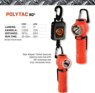
The solution to firefighters' hands-free lighting needs. Attaches easily to helmets and hard hats, and rotates 360°. Fits snugly against helmet to prevent snags. Features a bright taillight LED so you can be seen from behind even in heavy smoke. Easy to operate with gloves. Fits both traditional and modern helmets.
